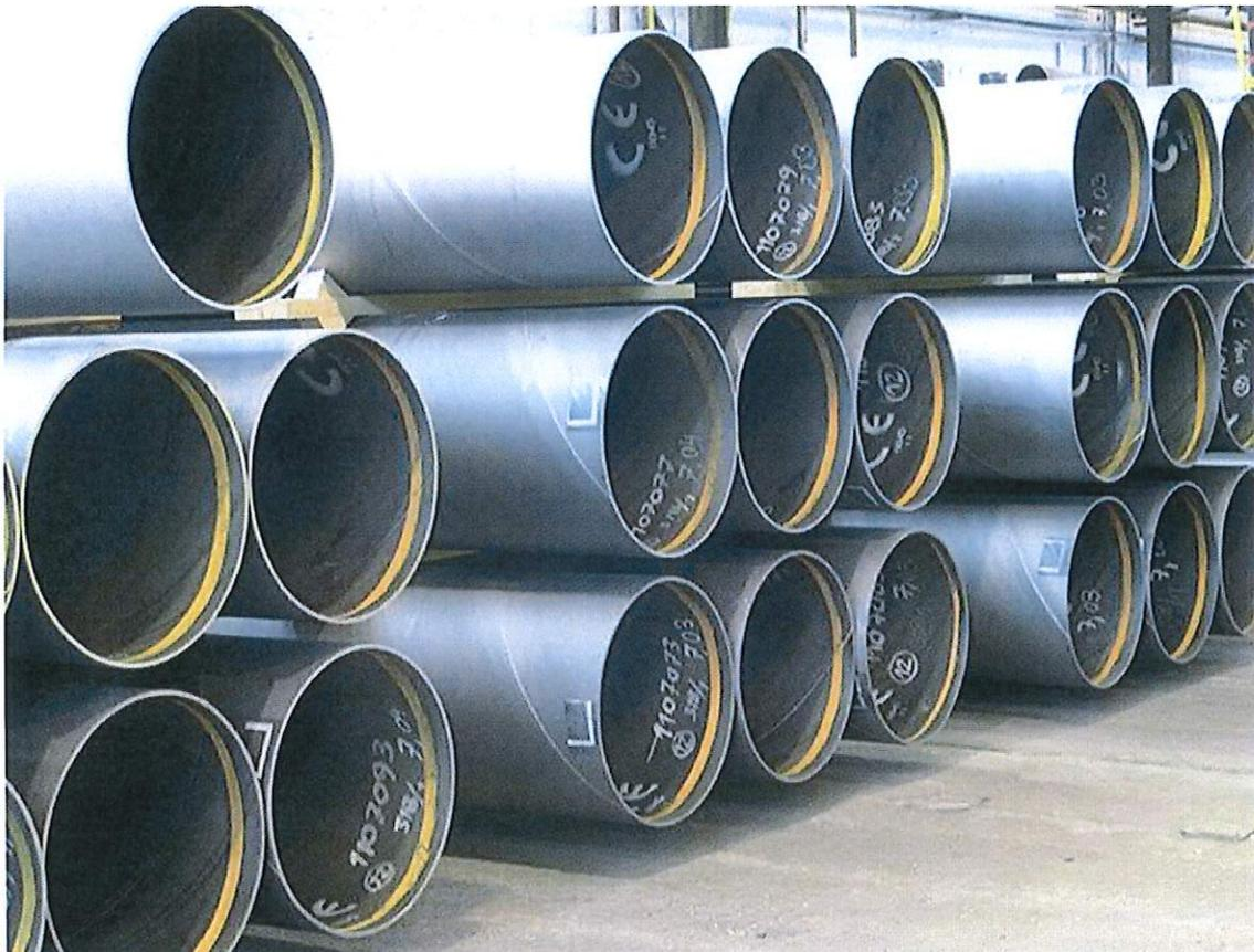
**Welded pipes (SAWH)**
